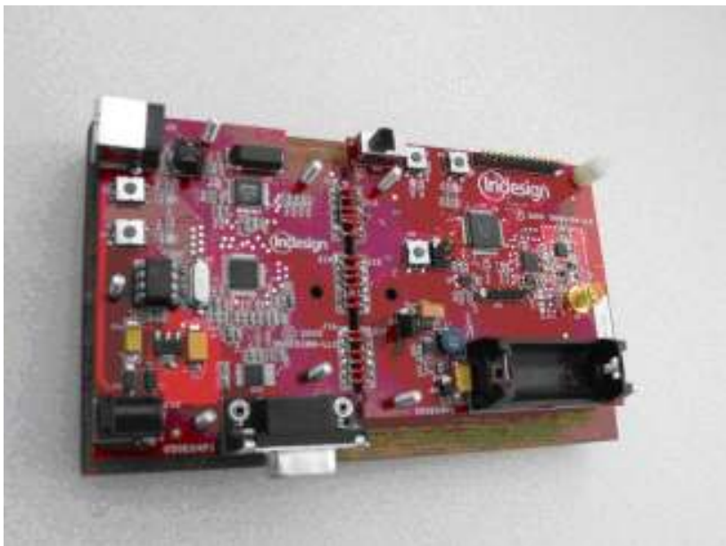
Figure 2: Sample ZigBee development platform including multiple command/debug interfaces, integrated sensors, GPIO access, with an integrated ZigBee radio chip.
